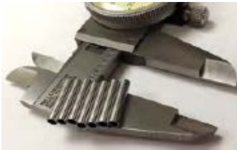
ECG for Burr-Free Tube Cutoff
