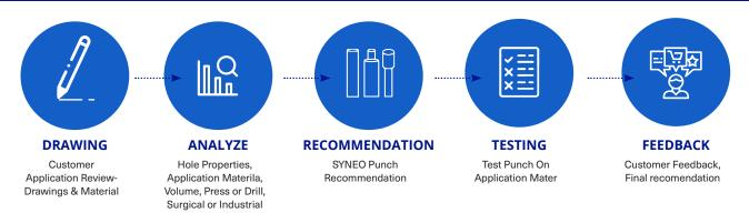
SYNEO's application review process is designed to ensure that customers receive proper hole outcomes with minimal iteration. SYNEO applications specialists review customer drawings and material properties to ensure that each cutting tool specified creates the desired hole on the first use.
