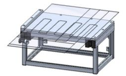
Adjustable Pouch Support Platform Assists in locating the pouch. Other Pouch Platforms can be designed on request.
