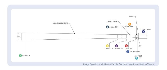
Both the P4K and the P5K, at both speed settings, measured the diameters (①,②,②) at a rate greater than 99 percent product variation, better than 0.000 012" or 2 percent of a .000 4" tolerance zone.
